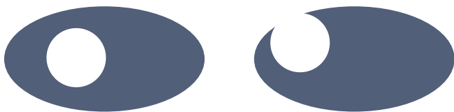
Figure 2.10-1: Left object includes one hole. Right object has no hole because the white area inside the object is not totally surrounded by the object
