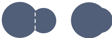
Figure 2.10-2: Left object is divided into two objects by the white boundary while the right object remains a single object when the Split touching objects processing is applied
